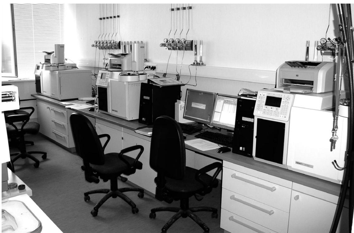
Gaschromatographic devices. Behind them on the wall there's the supply with industrial gases
