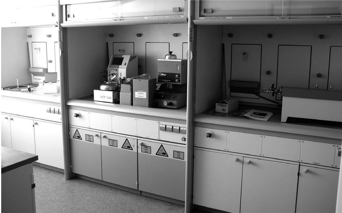
Exhausters with ash, flashpoint, micro carbon and evaporation residue devices
