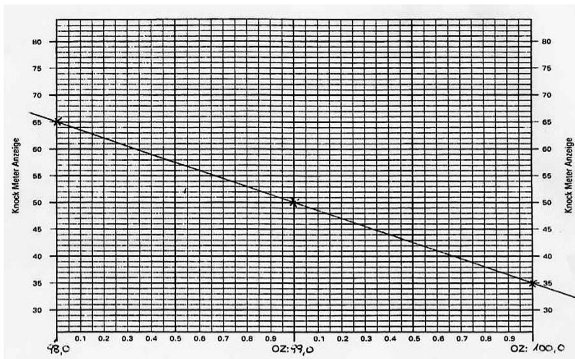
Diagram for the calculation of octane rating
